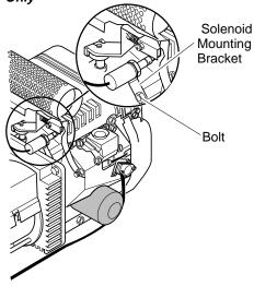
Figure 28 - Solenoid Bracket Location, Model RGH11000AIE Only
